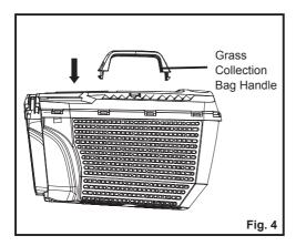
3. Align the cover and base of the grass collection bag at the front. Clip the two halves together, starting at the front and then moving to the sides (Fig. 5).
