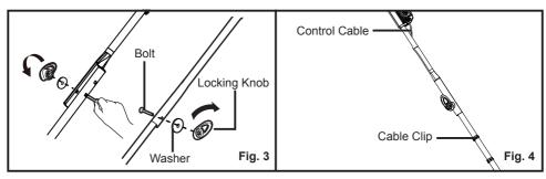
2. Secure the control cable with the cable clips (Fig. 4).
