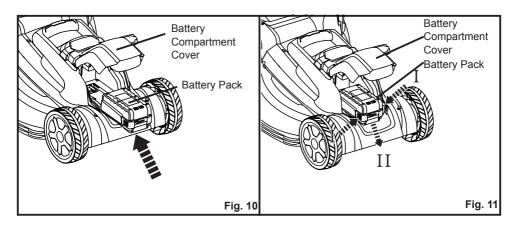
**NOTE:** Make sure that the battery pack firmly snaps into place and is secured to the mower before starting operation.
