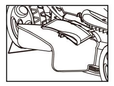
The mower is designed to disperse the clippings back to the lawn. Pull up the cover and insert the side discharge chute. The side discharge is optional, if you do not need the side discharge, remove from the mower.
