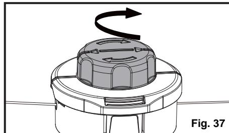
**NOTE:** Always clean the trimmer head cover and trimmer head housing before reassembling the trimmer head.
